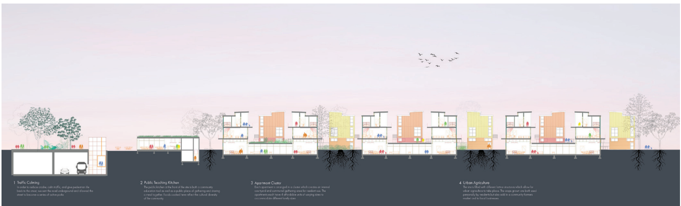
Figure 6. Submerging a main thoroughfare mitigates the health inequities caused by the high-crash corridor. Lorine Moellentine and McKenzie Vanko.
